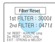
Primary filter reset – press and hold the button for more than 3 seconds or alkaline
