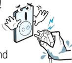
Ensure the power plug is firmly and properly inserted into the outlet – failure to do so may result in electric shock or fire!
