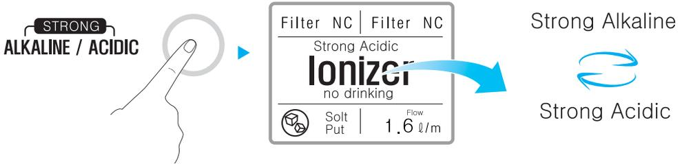
※After producing strong alkaline water/strong acidic water 30 seconds of cleaning job will be implemented before returning to the setting function.
