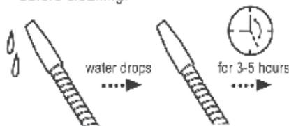
7. Turn on the Flow Control Valve until water drips from the Flexible Stainless Spout. Then turn off the Flow Control Valve and allow the ionizer to sit for 3-5 hours.
