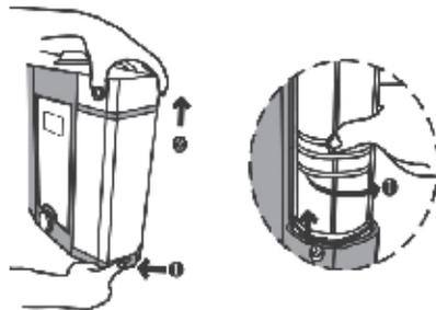
3. Open both filter covers and remove both filters.
